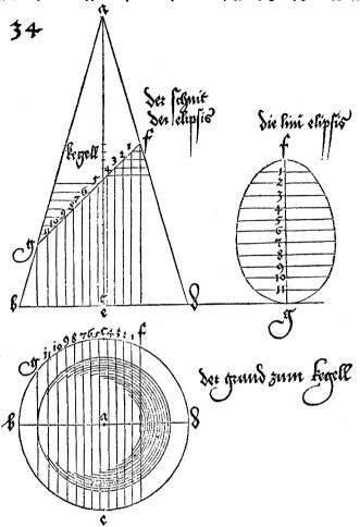
another then any convenient line can be used. This is the case in Dürer's drawing where the centre line of the circle is used as the reference line in the top view.
